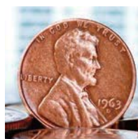
Oxidized: coated in copper oxide
